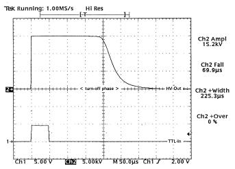
HTS 150 with 100 $\mu$ s on-time extension. R<sub>L</sub> = 1M $\Omega$ , C<sub>L</sub> = 20pF, vert. 5kV/div.
